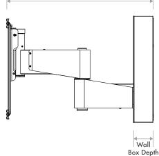
Height: 20.76" [52.7 cm] Width: 32.76" [83.2 cm] Total Depth: 4.44" [11.3 cm] Ext. Depth: 28.59" [72.6 cm] Wall Box Depth: 3.85" [9.75 cm]
