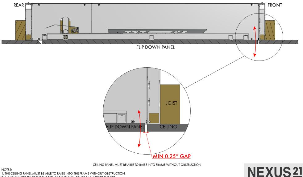
1. THE CEILING PANEL MUST BE ABLE TO RAISE INTO THE FRAME WITHOUT OBSTRUCTION 2. MANUALLY STOPPING THE FLIP DOWN PANEL WILL CAUSE DAMAGE TO THE LIFT
