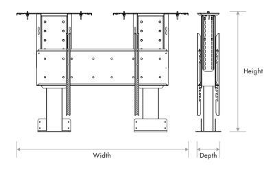
Height: 28.5" [72.4 cm] Min / 40.5" [102.9 cm] Max Width: 42" [106.7 cm] Depth: 5.375" [13.7 cm] back of TV to back of TV
